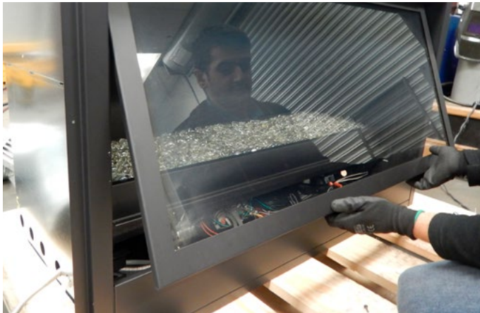
Figure 9: Remove the tool from the latch slot. Ensure the latches are hanging freely, the hook end is released from the bottom of the door. (Repeat all 4-steps for the remaining latch)
