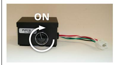
After 20 minutes of running turn speed control to the right, the motor speed will slow, keep turning the control knob to the right until the burner turns off.
