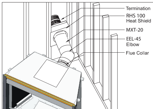
Figure 17. Corner installation (Rigid). (Natural Gas Models Only)
