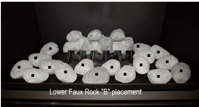
Figure 30b. Placement of (17) seventeen Lower "B" faux ceramic rocks. Note approximate location and placement. (Do not cover the burner holes if possible). (Place one of the rocks on top of the Pilot cover *).
