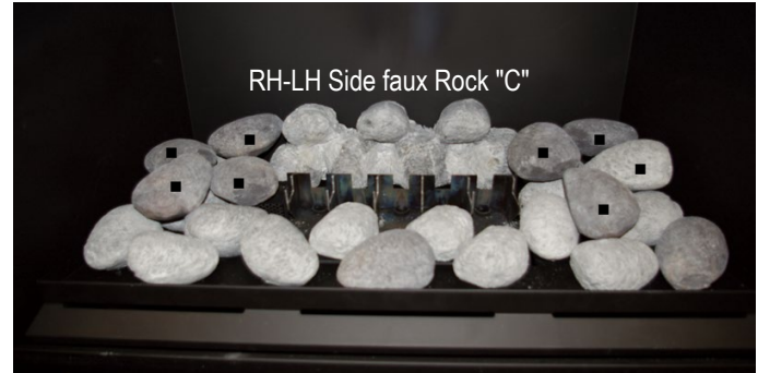
Figure 30c. Placement of (8) eight LH & RH Side "C" faux ceramic rocks. (Marked). Note: approximate location and placement. (Place on top, in between the lower layer rocks in a pleasing pattern).
