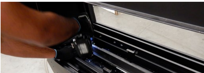
Figure 12.d Removing the Burner screws
