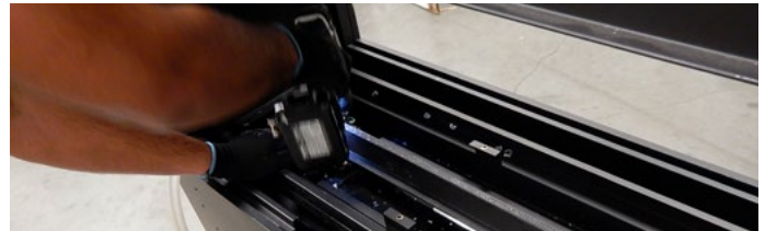
Figure 13. Removal of burner strip
