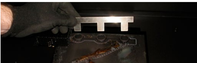
Figure 23.d Pushing the Rock Guard down into place.
