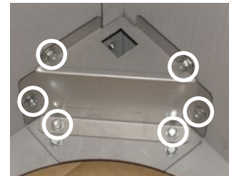
Figure 3.e Unscrewing control cable cover
