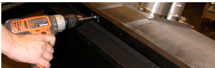
Figure 3.3 Fixation de la plaque coulissante
