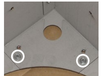
Figure 3.f Removing strain relief plate.
