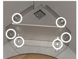
Figure 3.e Unscrewing control cable cover
