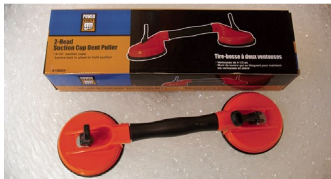
Figure 16d. Supplied Glass lifting tools.
