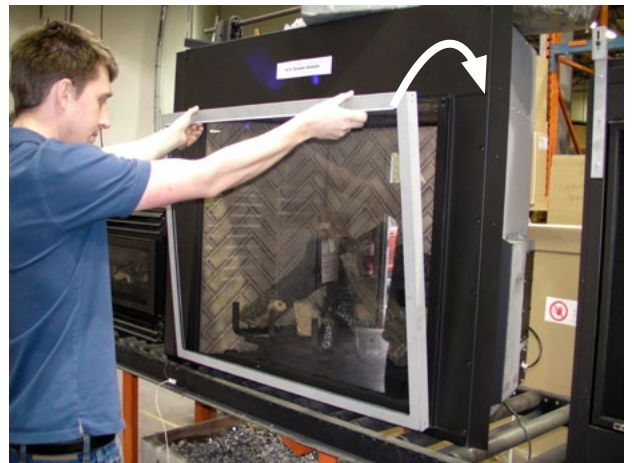
Figure 17d. Pushing screen into place.
