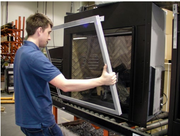
Figure 16b. Lift screen off retainer slides.
