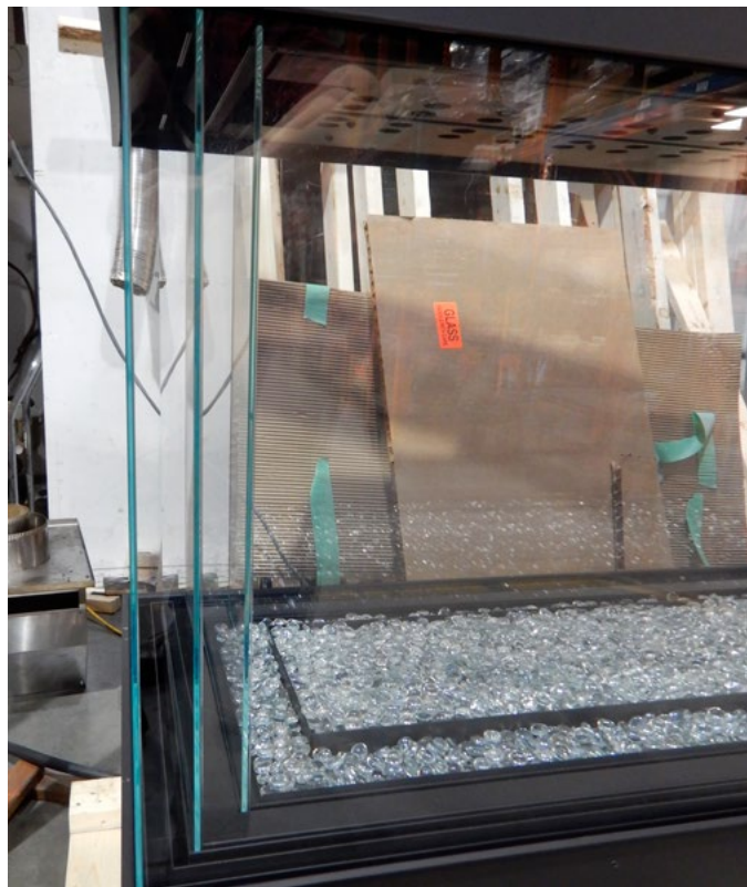
Figure 100. Glass installed (side view - no gaps)
