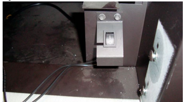
Figure 15 Attach switch to bracket.
