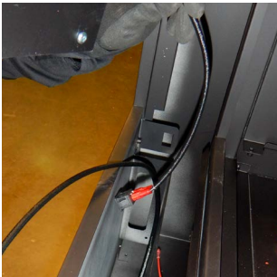
Figure 24.e On/Off switch through drawer
