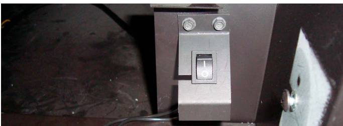
Figure 21 Attach switch to bracket.
